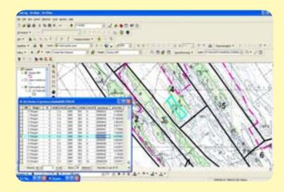
and data entering into field manuals, all data is transferred into the software package. In order to present results in the cartographic way, data can be exported into an appropriate Excel or Access base which is then connected with maps by the GISODSEK key.
